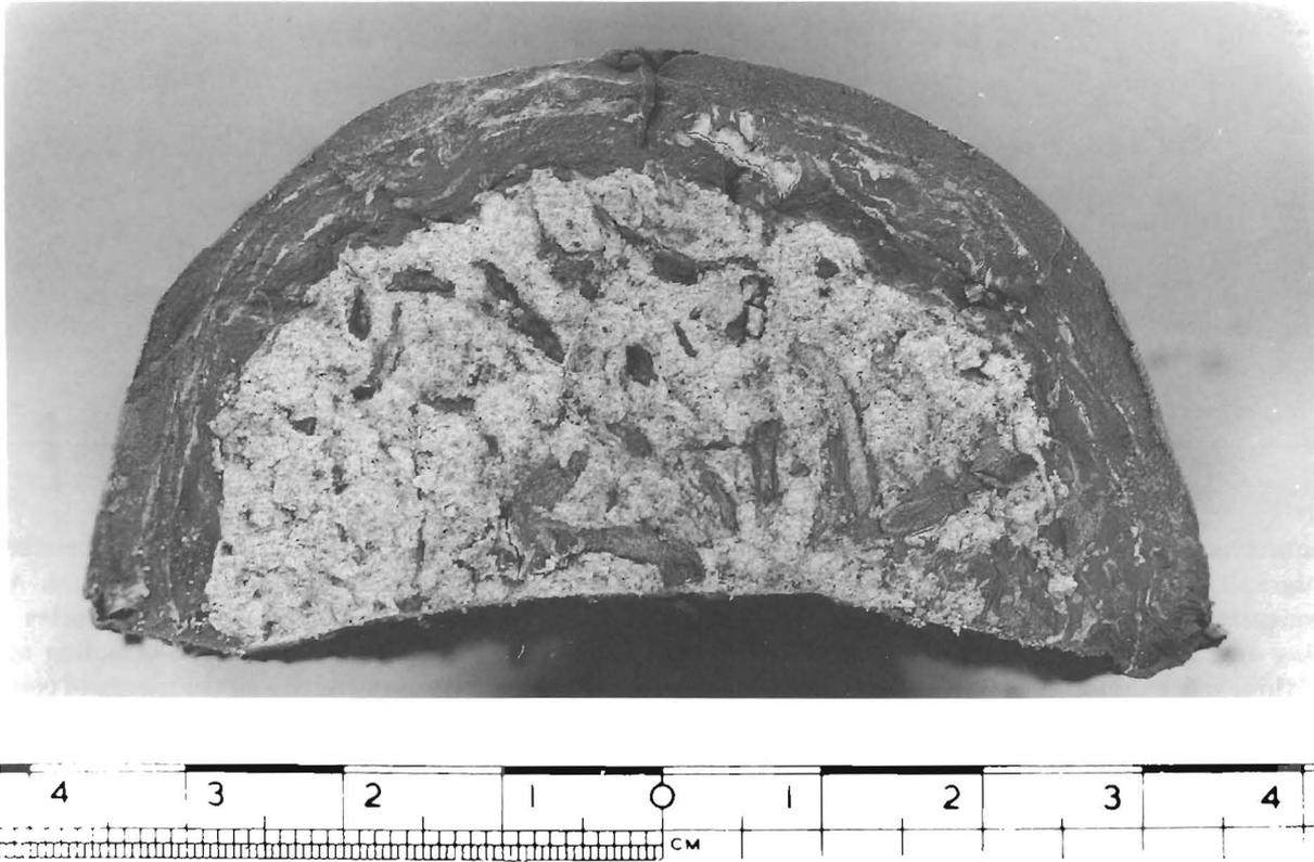
FIGURE 1. Photograph of horizontally split core section; vibrocore 51/07/199 from the central Celtic Sea. Scale intervals are 1 cm.
